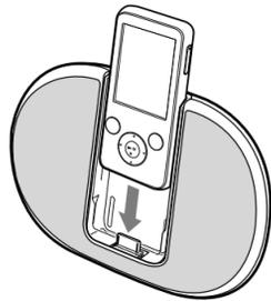
Make sure that the "WALKMAN" is placed properly in the WM-PORT of the system for proper connection.
