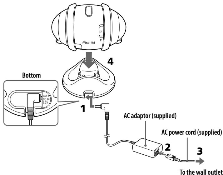
**1** Connect the AC adaptor to the DC IN 5.2V jack of the cradle.
