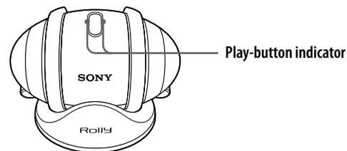
The Play-button indicator of Rolly lights up in orange, and charging of the battery in Rolly starts.
