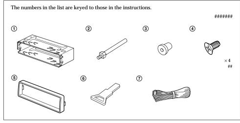
The release key **(6)** is used for dismounting the unit. See the Operating Instructions manual for details.
