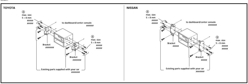
Note To prevent malfunction, install only with the supplied screws (4).
